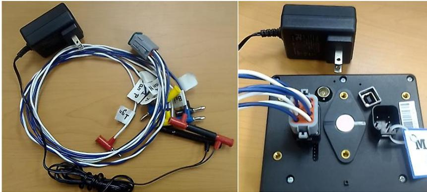
2. Connect the unit the computer through the debugger. This will be done using the **ST-LINK/V2 Debugger Connections into a maxAI 430 with SDK Code manual** provided alongside this guide. See the figure below to verify the pinout:
