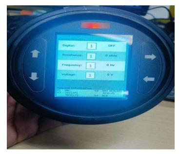
The configurable input is designed to configure various input channels. It is used to update the latest configurable input values based upon the previously configured channel properties. The different configurable inputs that are currently available are Digital, resistance, voltage and frequency. The blocks in the figure represents different configurable inputs.
