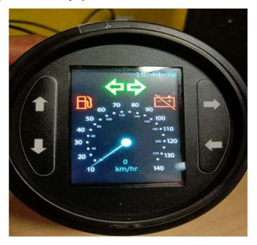
In the above image all the sections of the screen are shown using the arrows, as each section is functioning for different test case such as RTC is for time, J1939 for Engine Speed.
