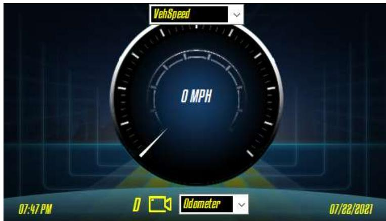
Single layout contains one analog gauge, that can be assigned to any of the **Gauge Sources** using the dropdown menu at the top of each gauge.
