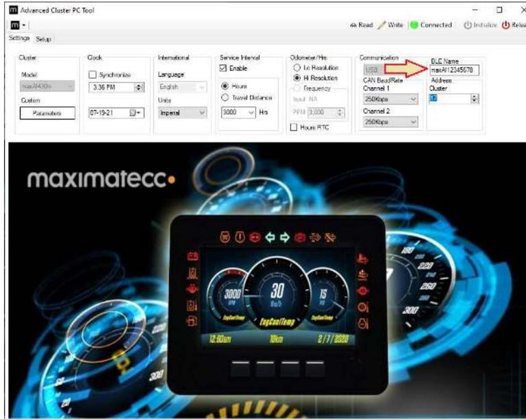
Before making a USB connection, you may wish to change the **BLE Name** (Bluetooth Name) of the device. In order to change the name of the device, you will need to initially connect via USB. Once USB communication is established, rename the BLE Name to desired designation.
