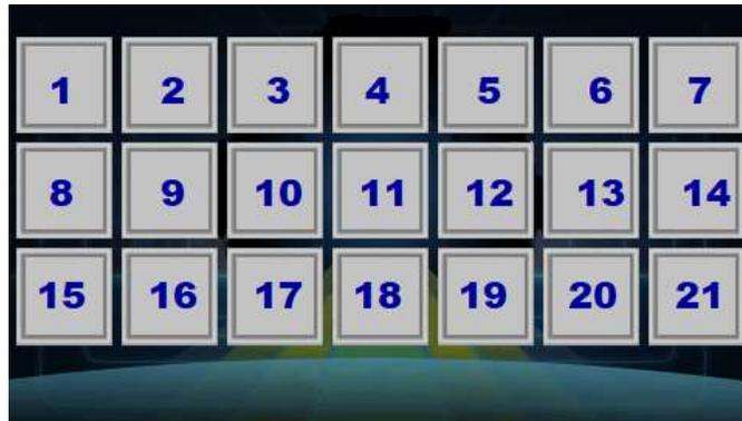
There is a total of 21 configurable LCD Warning Lights. Editing capabilities for warning lights are the same as for the gauges.
