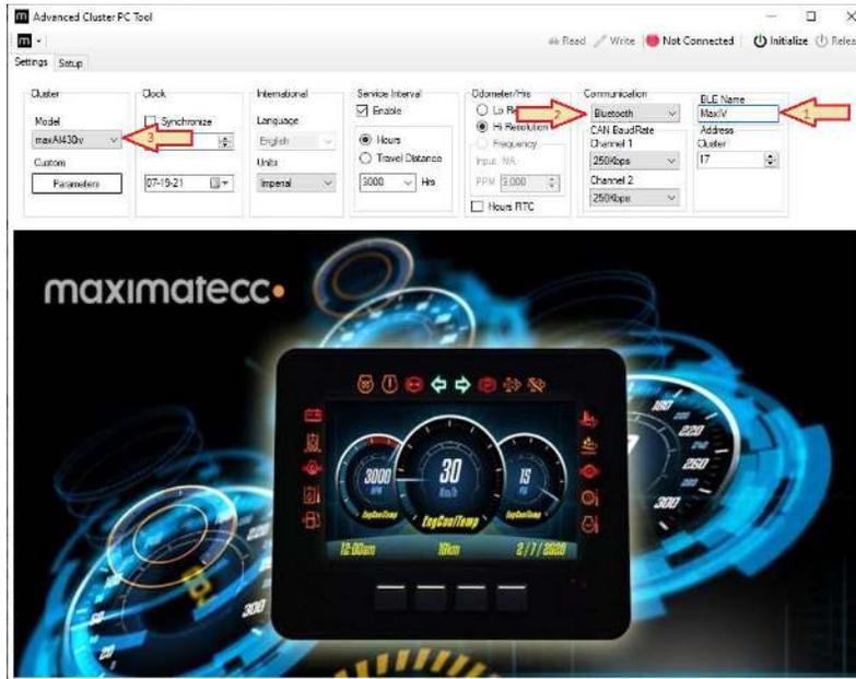
Once the BLE Name is known you are ready to connect via Bluetooth. To connect, first make sure the BLE Name is correct to match the device you wish to connect to. Once the BLE Name is correctly filled in, select the model being connected then selecting **Bluetooth** under **Communications**.
