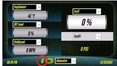
This option will enable the cluster to display the transmission gear position (current gear), once this option is enabled the display will show the gear information at the bottom of the screen by using the current gear J1939 SPN from the transmission source address.
