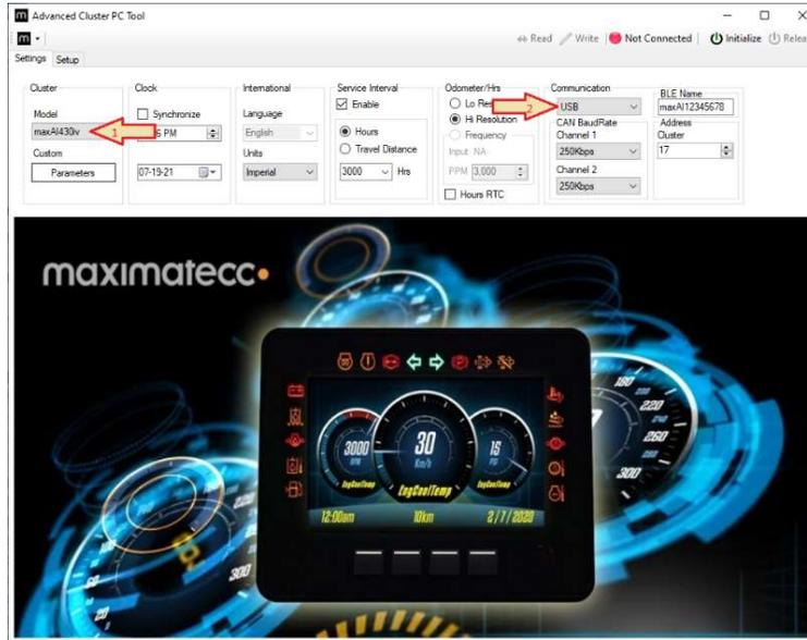
After connecting all hardware with a USB cable and opening Configuration software, establish USB communication by first selecting the model being connected then selecting **USB** under **Communications**.
