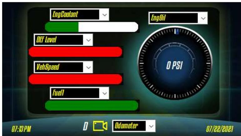
Analog layout contains four bar gauges and one analog gauge, that can be assigned to any of the **Gauge Sources** using the dropdown menu at the top of each gauge.
