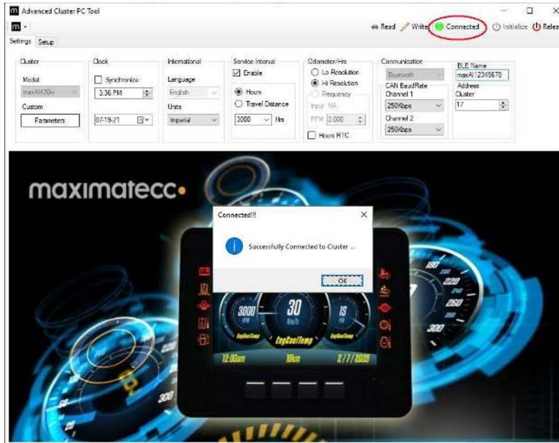
Once communication is established, a pop up will confirm successful connection to the device and the Config Tool will indicate that it is connected at the top of the window.
