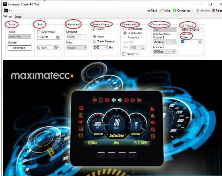
**Cluster Parameters** menu allows you to view and adjust communication parameters for specific models.
