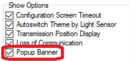
This option will enable the cluster to display to report fault codes received from Engine, Transmission or Retarder. The fault codes notice will appear as a banner in the top of the LCD screen.
