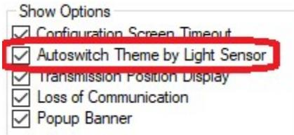
This option will enable the cluster to automatically switch between Daylight or Nighlight color themes. When disabled the color themes should be manually selected by user using the Configuration Screen menu.
