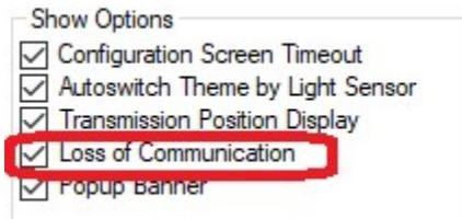
This option will enable the cluster to report the CAN communication loss for any of the two Channels. The CAN loss notice will appear as a banner in the top of the LCD screen.
