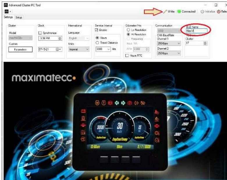
Once the BLE Name is filled in, select **Write** to set the new BLE Name to the device.
