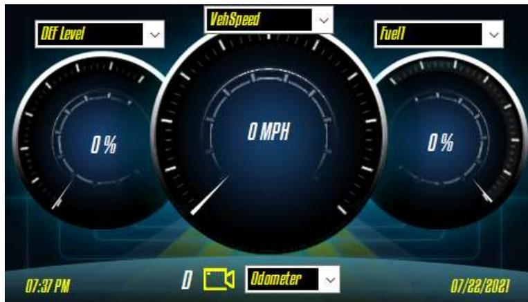
3 Gauge layout contains three analog gauges, that can be assigned to any of the **Gauge Sources** using the dropdown menu at the top of each gauge.
